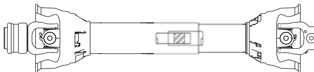
End Yokes Properly Aligned
